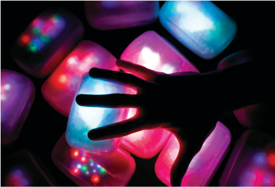
Figure 5. Translucent acrylic cases fitted with 20 colored and white LEDs each, a microphone and a vibration tab, which allow people to modify their personal “lightscape.”
