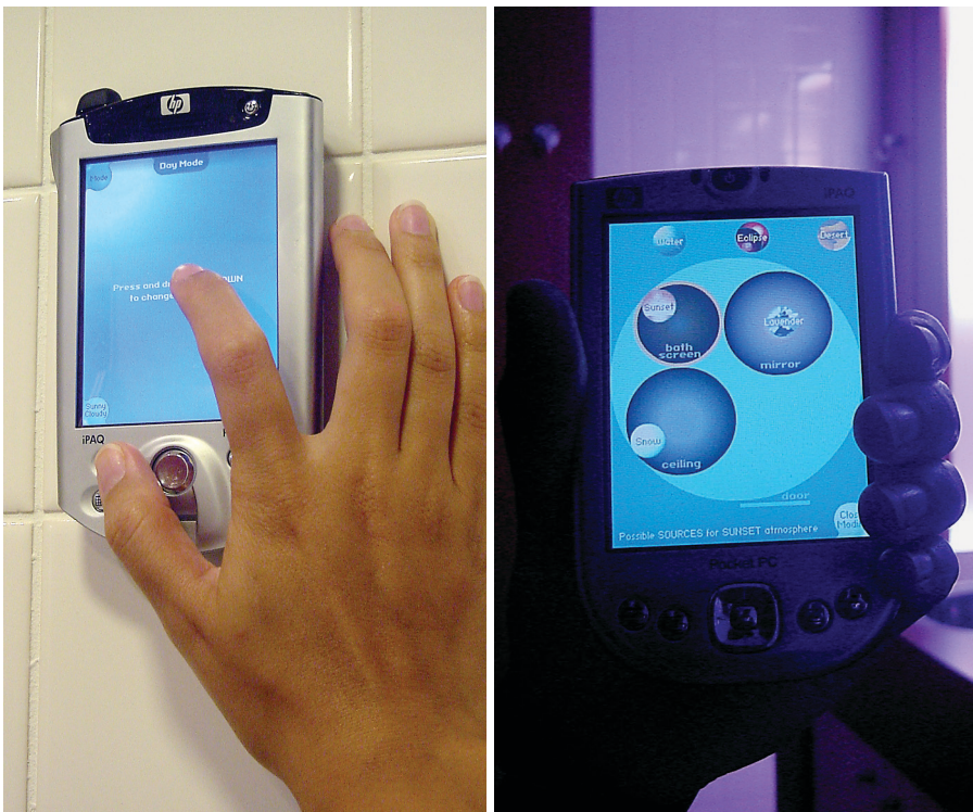
Figure 3. A light switch using a handheld mobile device to control groups of warm and cold white light (left), and to spatially position and dim groups of colored lights (right).
