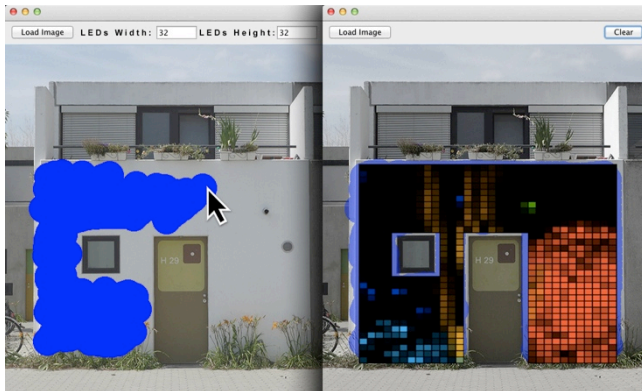
Figure 5. The Mapping Tool helps defining a non-rectangular screen based on architectural images and models.
