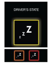
**Figure 1:** An *on-time warning* is displayed when a critical value is reached (here: drowsiness). A warning features a color-coded frame indicating the urgency.
