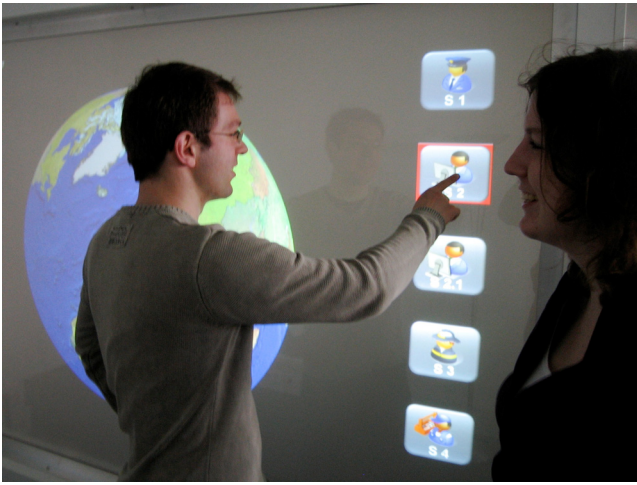
Figure 1: Multi-user interaction with a multi-touch wall in an emergency scenario without dedicated access control: The user is selecting an authentication level by pressing a button representing a certain role.
