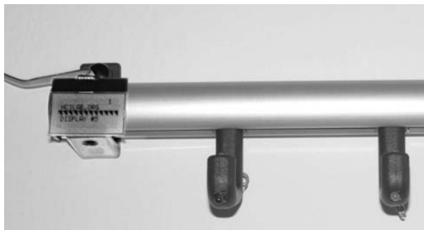
Figure 5: Graphical display, LEDs, and sensors included into a coat hanger as embedded weather display.
