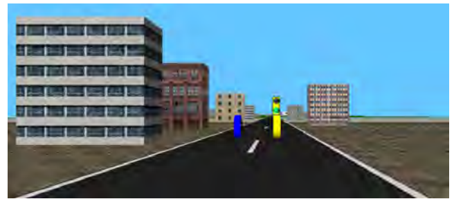
Figure 1: A screenshot of the ConTRe . The driver controls the movements of the blue cylinder while the yellow cylinder moves autonomously.
