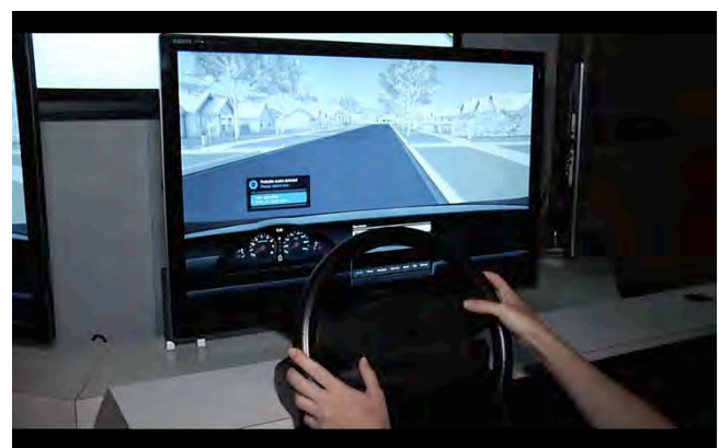
Figure 1. Interactive Demo Presentation at Research @ Intel Days. LCD TV simulates HUD notifications, while gesture pad embedded in upper right steering wheel spoke enables gesture interaction with the HUD.
