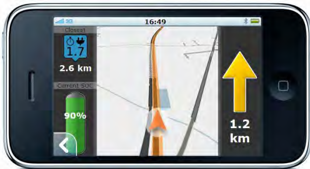
Figure 7: Traditional navigation leads to the charging station while the distance of the closest charging station is shown.
