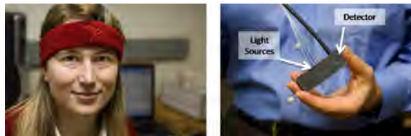
Figure 1. Two fNIRS sensors (right) are attached under a headband (left). There are four near-infrared light sources and a light detector on each sensor.
