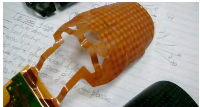
Figure 5. Capacitive film from off-the-shelf mouse
