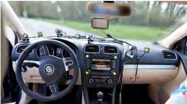
Figure 2: Volkswagen Golf VI cockpit equipped with mobile navigation system and eye tracker.
