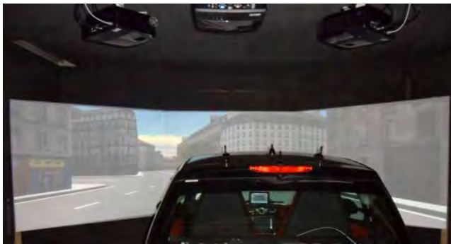
Figure 2: The lab setting on Saarland University Campus. Fixed-base simulator running OpenDS with three projectors (120 degrees field of view) and connection to CAN-bus.
