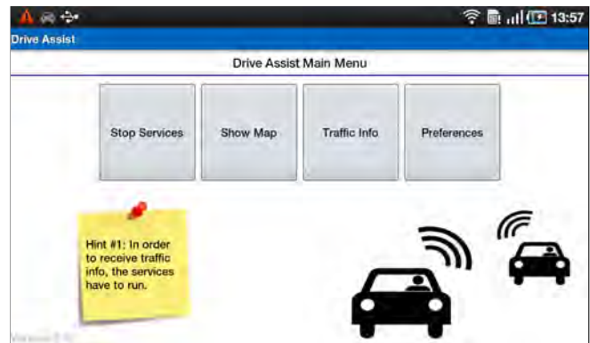
Figure 1. The main screen of DriveAssist research prototype. The yellow sticky label-like box in the lower left corner shows random hints for the user. In a first user study, only one out of 12 participants found this way of providing hints useful.
