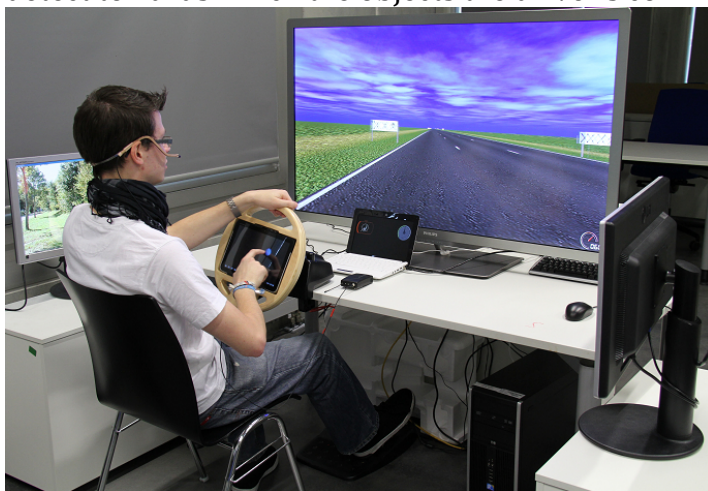
Figure 5: A second prototype of a multi-touch enabled steering wheel was used to test the multimodal combination of gestures and speech.
