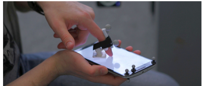
Figure 1. A participants performing 32.5° pitch and 45° yaw with the left hand while being equipped with our 3D printed tracking parts.
