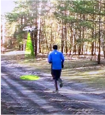
Figure 1: Pathfinding using a light cone emitted from a drone while a runner follows through a forest (Image source: [14]).
