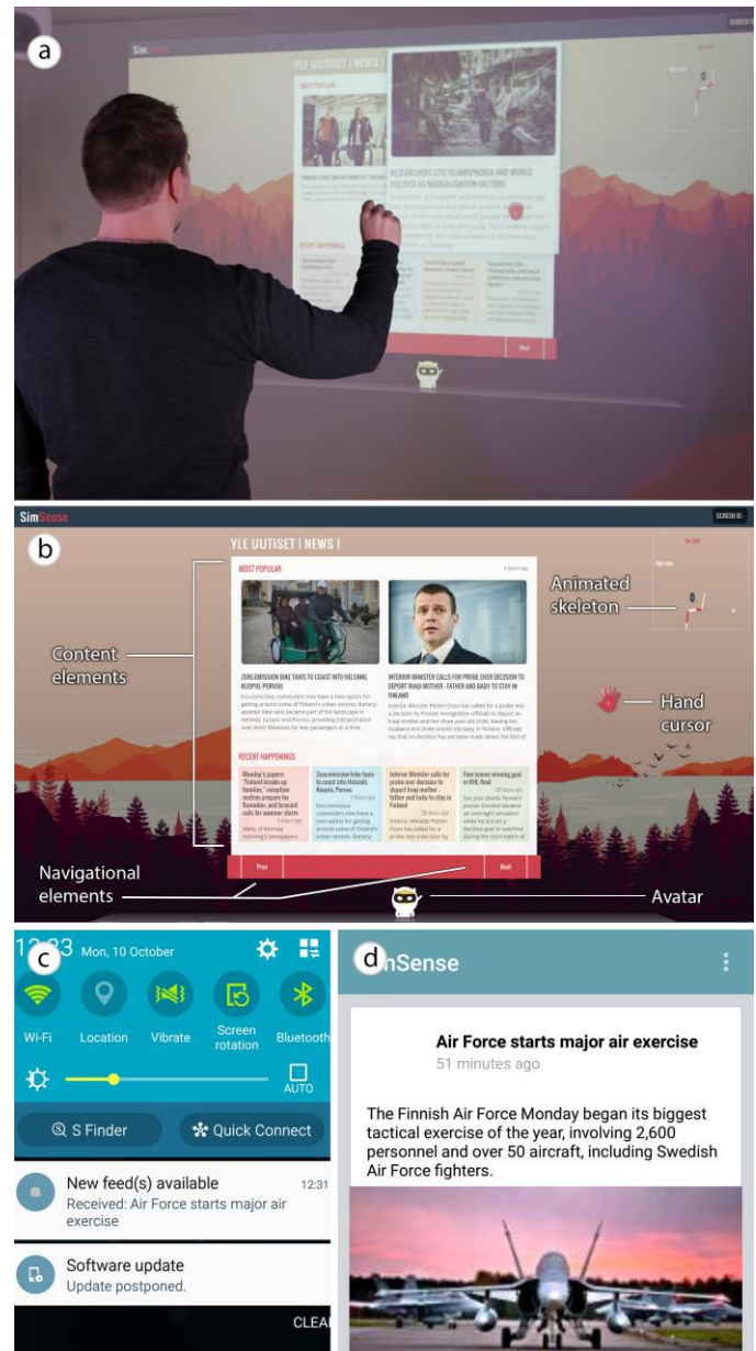
Fig. 1. A) A user is transferring content from the large information display to his mobile device by performing the grab-and-pull gesture. B) An overview of the elements in the large display application. C) “New feed(s) available” notification on the mobile device about received content. D) The SimSense mobile application displaying content that was transferred from the large display.
