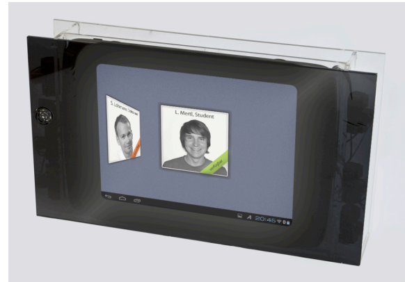
Figure 1. Prototype of a gesture-controlled information display which can be placed next to office doors.
