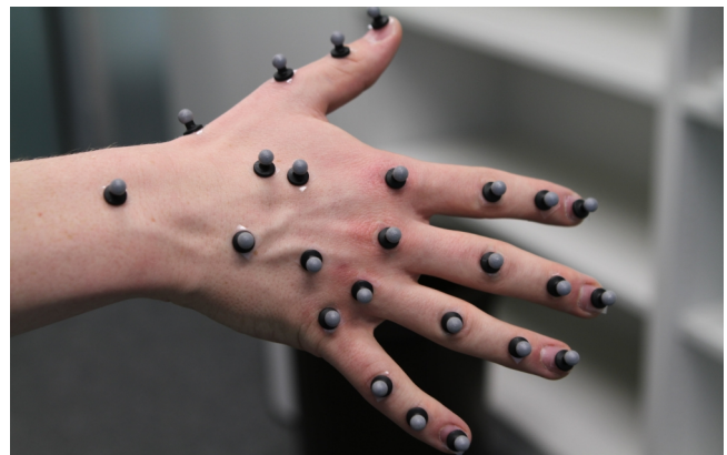
Figure 3: Placement of the reflective markers (6.4 mm spheres) on the right hand for enabling motion tracking.
