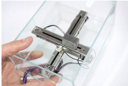
Figure 2 Two-dimensional weight-shift-based haptic display; Weight-Shifting Mobiles prototype.
