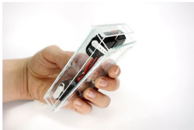
Figure 1 Shape-based display of digital contents in mobile phones; Prototype from the Shape-Changing Mobiles
