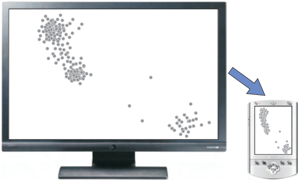
Fig. 1. Example for lost effectiveness of a conventional scatterplot due to transfer to a smaller display: the perceived number of classes may change from three to two.
