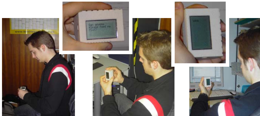
Fig. 3. A typical scenario in the user study: First the tester sees that there is a new message, picks the display up and reads the message. To answer the questions he tilts it correctly to the left, but in a way that he can no longer see the contents of the display. However, he soon recognizes that he can hold it comfortably in a way that he can read his answer.
