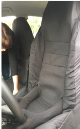
Figure 2: Ghost Driver: special car seat costume introduced by Rothenbücher et al. [16, 5] to facilitate Wizard-of-OZ field studies involving autonomous vehicles (Image credit: [16, 5]).
