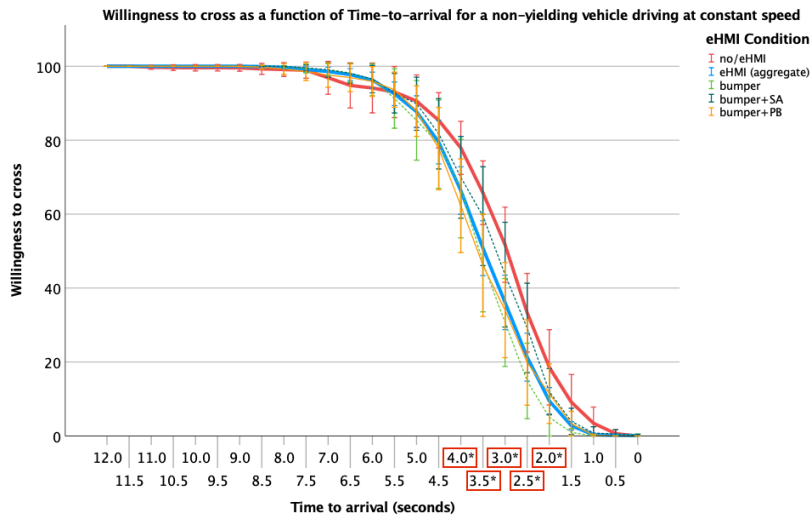
(a) The variation of pedestrians' willingness to cross as a function of the time-to-arrival for a non-yielding vehicle driving at constant speed of 50 km/h.
