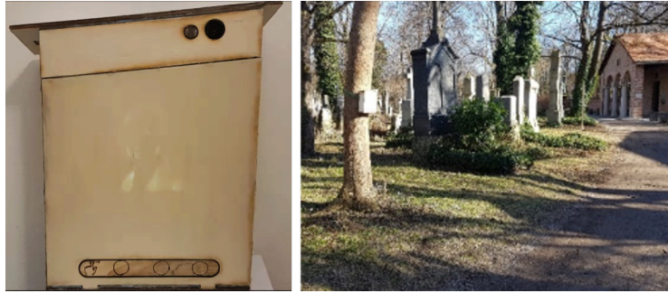
Fig. 2: Left: The birdhouse-inspired mid-fidelity prototype can display text via an LED matrix connected to an Arduino UNO triggered by four touch buttons. A portrait of the person is carved into the wood from the backside. When somebody approaches the object, an ultrasonic distance sensor triggers its illumination from behind and makes the portrait appear on the translucent wood. Right: The prototype in context.
