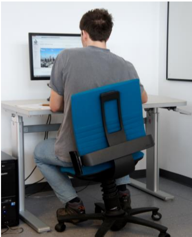
Figure 1. Users controlling a desktop computer through the movements of their body, while sitting on a sensor-equipped flexible office chair.
