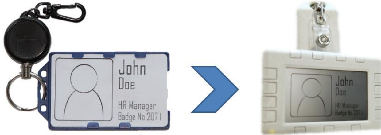
Figure 2: A traditional Badge with retractable string (left) and Interactive Belt-Worn Badge with an augmented retractable string and a display in the form factor of traditional badges.
