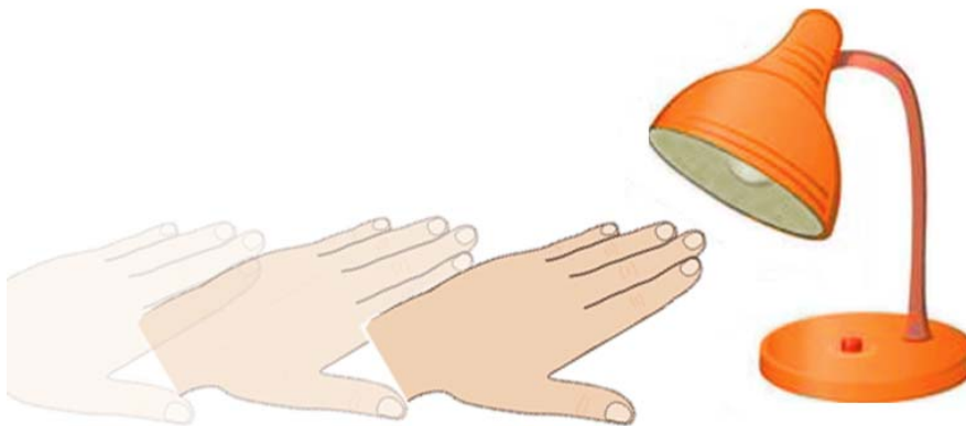
Fig. 1: Turning on the light by simply reaching towards the lamp
