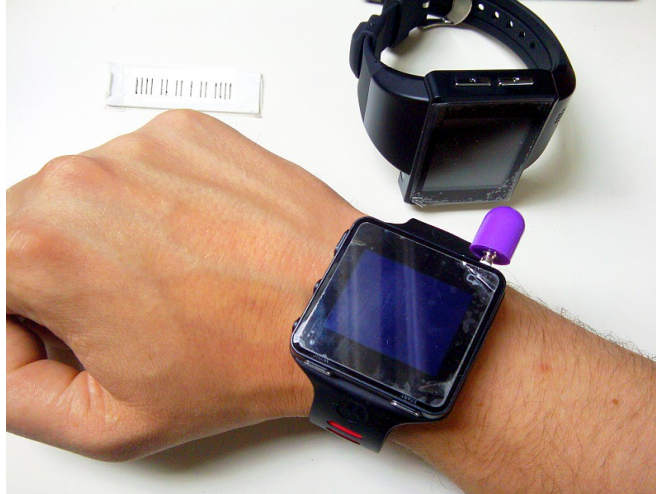
Fig. 1. Prototype using acoustic bar codes (top left) and smart watches equipped with a camera (top right) and microphone (bottom)
