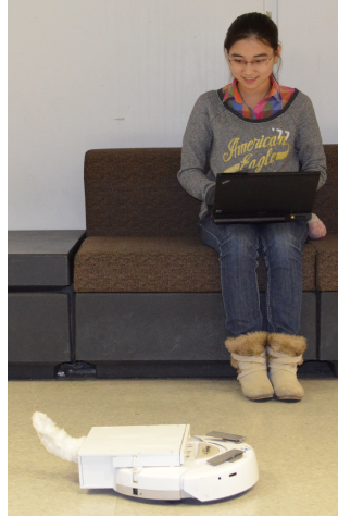
Fig. 1. A person notices the ambient tail state of a cleaning robot
