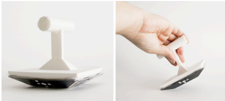
Figure 3. Graspable device equipped with markers: To interact, participants tilt the device, which subsequently moves back to its initial position on its own.
