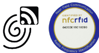
Figure 4.15: On the left the NFC-symbol indicating that it covers a Mifare Standard 1k NFC-tag as seen on the right.
