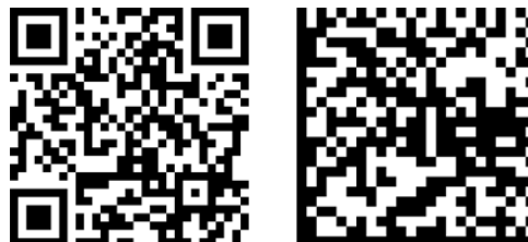
Figure 2.1: Examples for visual markers. The left one is a so called QR Code while the right one is a Semacode [19]. Other visual markers do exist.
