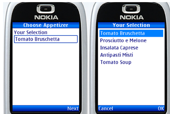
Figure 4.14: The rather uncommon but standard behavior of radio buttons using J4ME.
