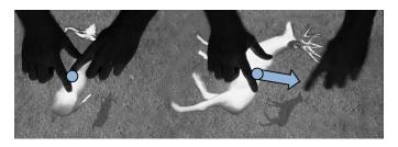
Fig. 2: Rotation technique described by Hancock et al. [9]. Flips a virtual object about the axis described by the first two touch points.
