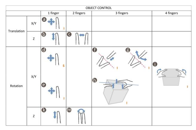
Table 1: Existing techniques for object manipulation. I: Integrated, S: Separated
