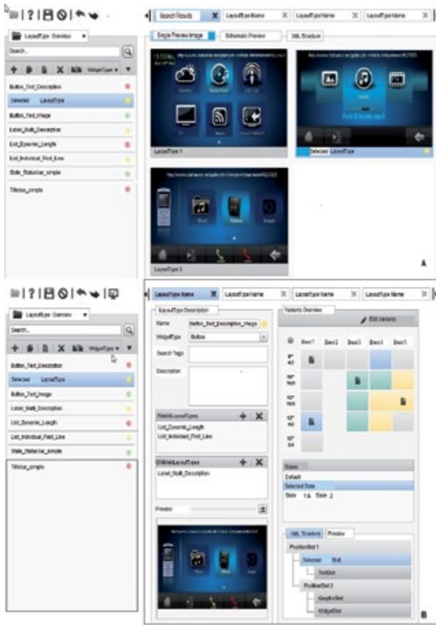
Figure 2: User Interface showing two different modes. A depicts the search mode for layout templates or variants. B depicts the layout template mode.
