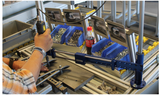
Figure 2. A state-of-the-art assembly workplace that is used in the analyzed sheltered work organization. Pictorial instructions above the boxes which hold the parts to assemble show how the assembly has to be performed. Workers can compare their assembled product with the depicted instruction.
