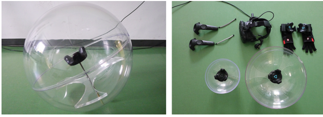
Figure 2: For the purpose of tracking two differently sized acrylic glass spheres (diameters: 25cm and 40cm), a threaded rod with stabilization had to be fixed to the spheres so that a tracker could be mounted in the center. The complete hardware setup consisted of a total of four trackers, a VR headset, tracking gloves for selection, and two controllers. All components are commercially available.
