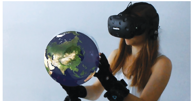
Figure 1: We show how a fully tangible spherical object can be utilized in VR by tracking an acrylic glass sphere with commercial hardware. This allows for the examination of the effects of a topologically equivalent tangible proxy object (image captured with Microsoft HoloLens).
