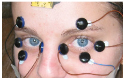
Figure 4: Sensors attached at the skin around the eyes (taken from [ metrovision@ ])
