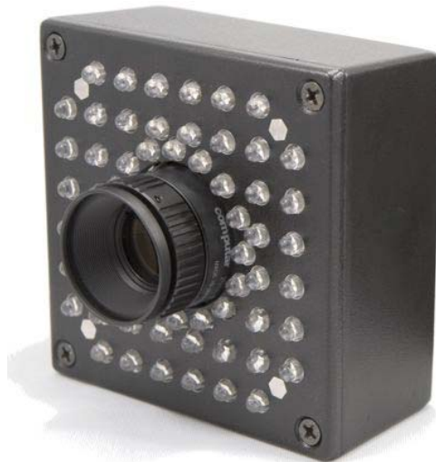
Figure 11: The Eye Contact Sensor Eyebox2 from xuuk inc. (taken from [ xuuk@ ])
