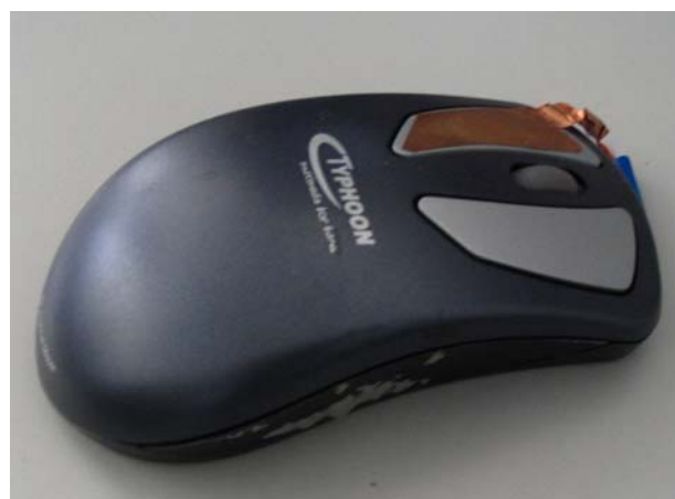
Figure 44 (right): The second version of the touch-sensitive mouse
