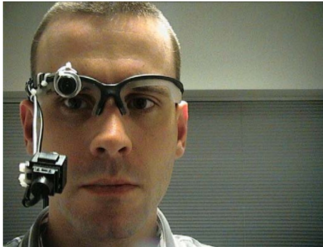
Figure 7: The Low-Cost Mobile Eye Tracker from the openEyes project
