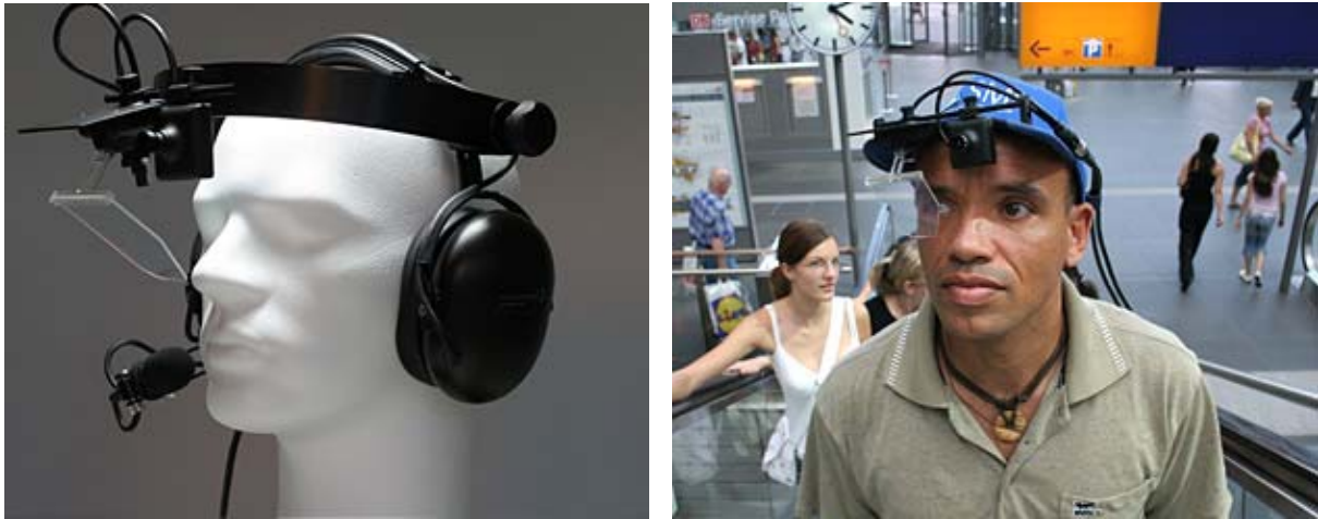
Figure 10: Head-mounted eye tracker from SMI (taken from [ SMI@ ])
