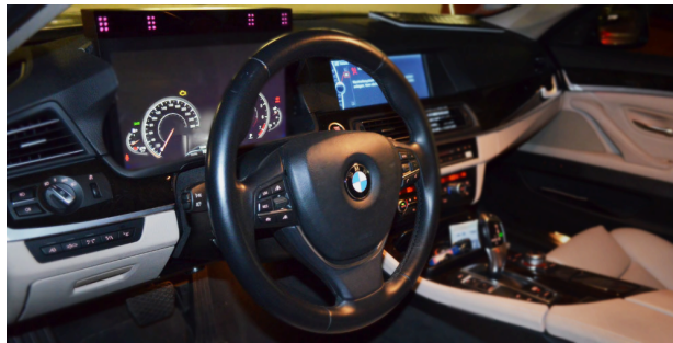
Figure 1: Test vehicle with an autostereoscopic display showing the instrument cluster.
