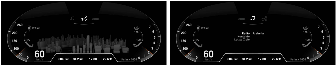
Figure 4: The driver can toggle between different views in the center of the IC. The left picture depicts a 3D map and the right the infotainment menu.
