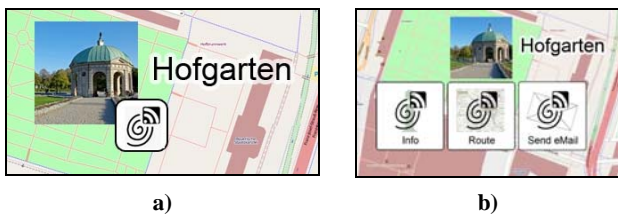
Figure 8. NFC-tags to select objects for further interaction (a) and to apply actions to individual objects instantaneously (b)
