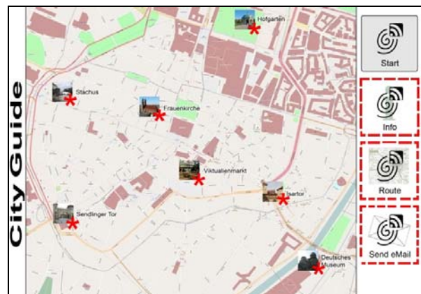
Figure 6. Physical UI for the combination of actions and objects. Asterisks and dashed boxes mark the positions of NFC-tags for objects and actions on posters for different prototypes (map from www.openstreetmap.de )
