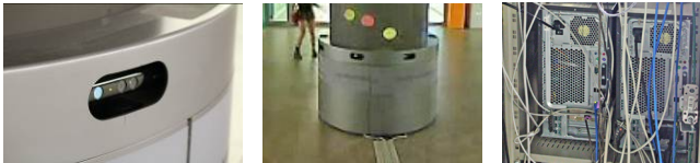
Figure 3.8 Kinect sensors integrated into the housing provide a seamless interaction space around the column, PC hardware runs the distributed Multi-Kinect application for our study.
