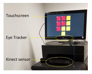
Figure 3.5: Technical setup for the study
