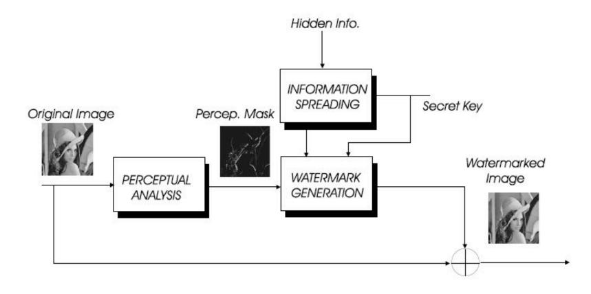
Figure 1: Watermark insertion unit
