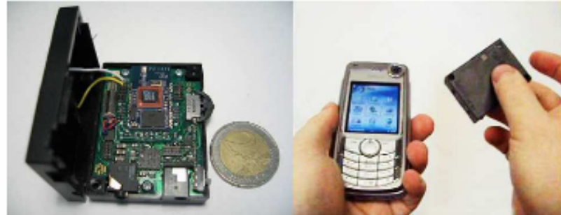
Figure 2. The wireless SHAKE sensor, shown with a 2 Euro piece for size comparison. This Bluetooth device comprises a complete inertial sensing platform.
