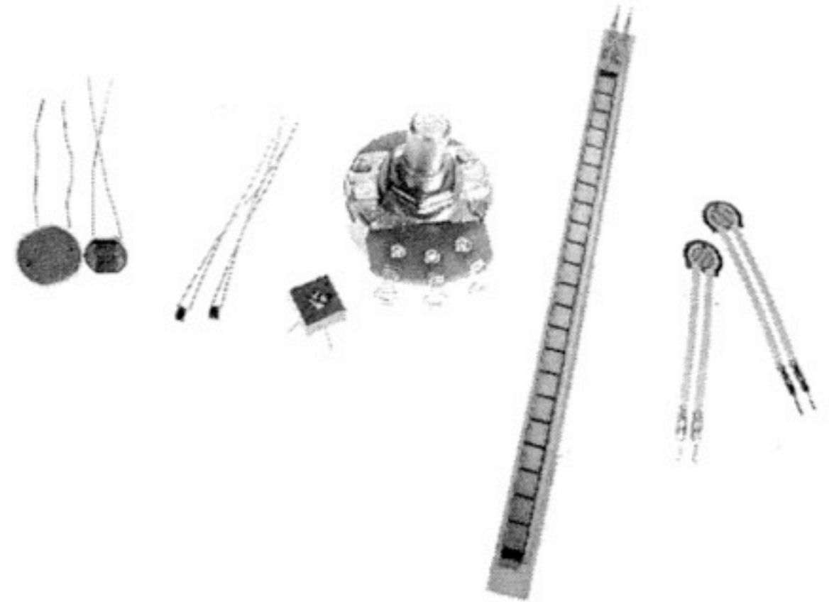
Figure 2.3 Variable Resistors. Schematics from left to right: generic variable resistor, photocell, thermistor, potentiometer. Images from left to right: photocell, thermistor, potentiometer, flex sensor, force-sensitive resistor (FSR).
