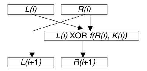
Encoding and decoding algorithms identical
