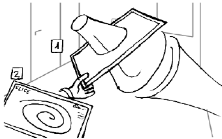
Figure 11. For scientific visualization the PIP can be used to specify and edit cutting planes ...
