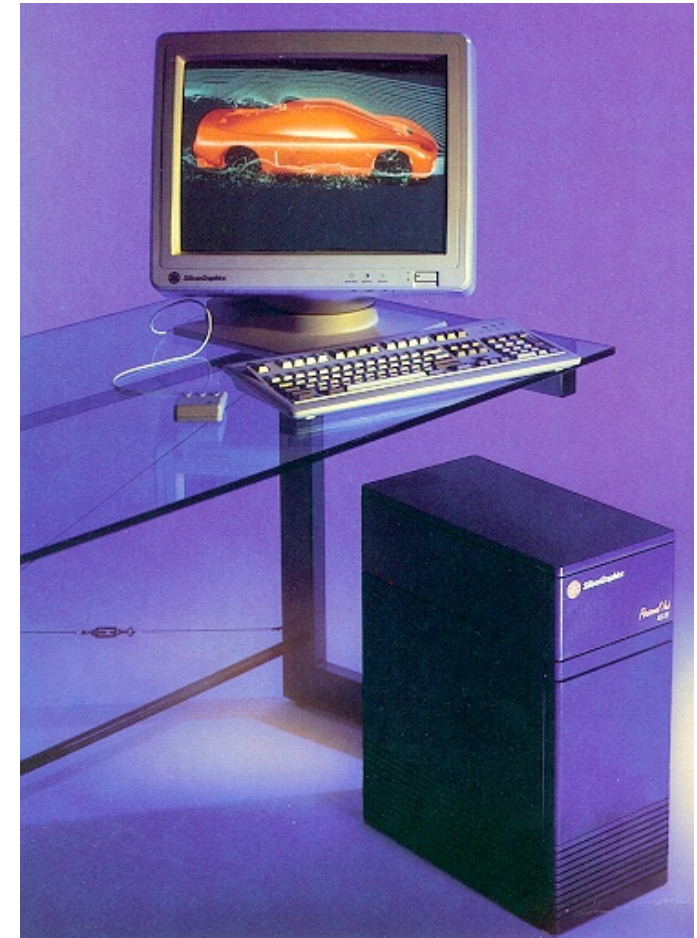
SGI IRIS 4D/35 (1991) 35 MHz CPU (RISC) Up to 128 MB RAM
