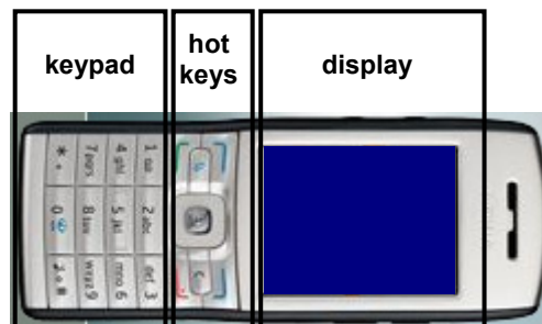
Figure 2: Regions of a standard mobile phone: keypad, hotkeys, and display. The S_{Micro} operator measures eye movements between those regions.
