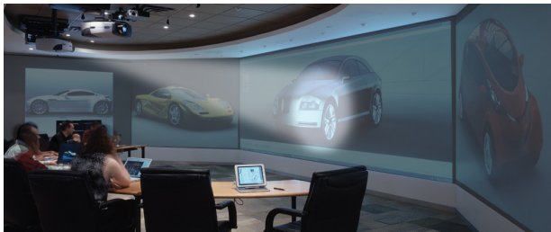
Fig. 3. Spotlight helps to draw the user attention to the required region of the wall sized display, meanwhile obscuring the remaining region to avoid distraction [19]
