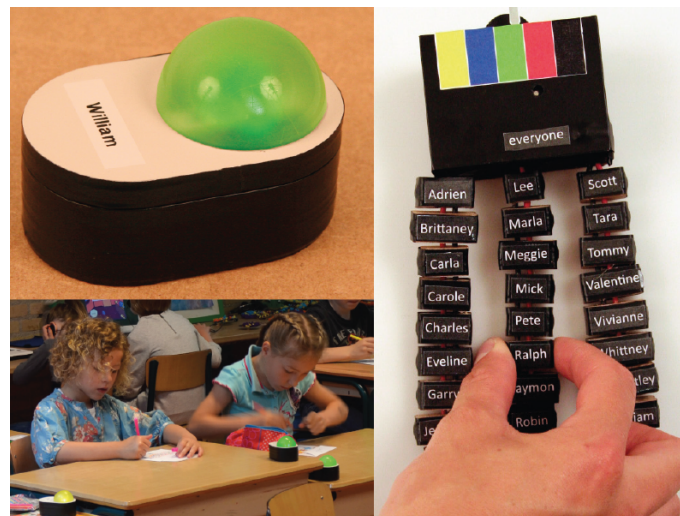
Fig. 5. The prototype of FireFlies consists of an ambient information component (left), that informs the students and let the teacher communicate with the students, and an peripheral interaction component (right), that enables the teacher to set the color of the students' ambient devices [1].
