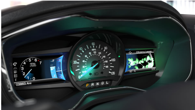
Fig. 6. Efficiency leaves in the 2014 Ford Fusion Hybrid SE [8]
