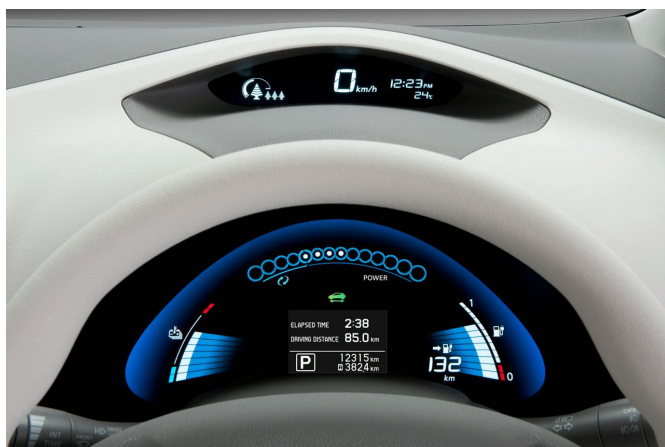
Fig. 4. The real time eco-Feedback display in the 2010 Nissan Leaf [23]
