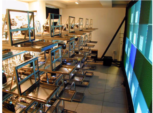
Fig. 7. A behind the scene photograph of the princeton scalable display wall , showing the array of 24 microportable projectors [9]
