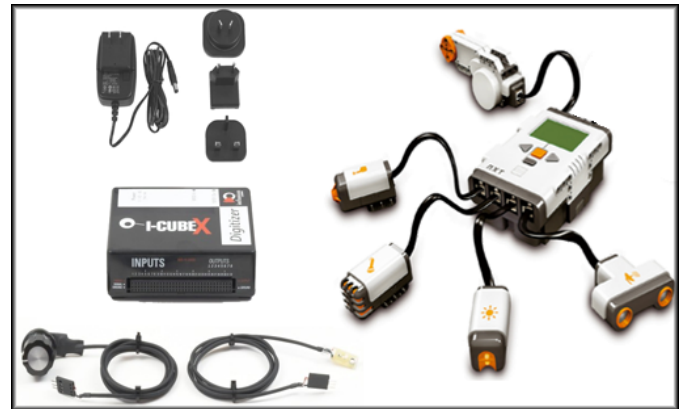
Fig. 3. a) I-CubeX toolkit b) Lego Mindstorm NXT 2.0; Sources: [1], [21]
